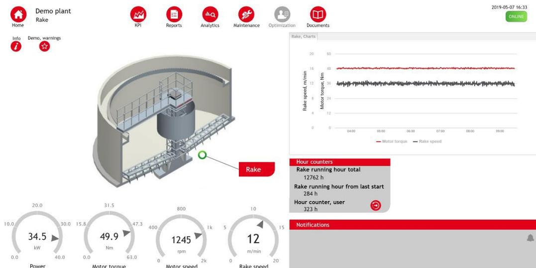
Figure 6. Thickener monitoring at mine in Finland.
