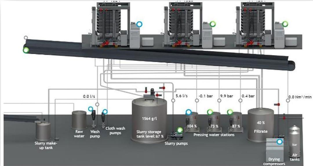
**Figure 4.** Depicted above is the digital twin image along with all the auxiliary equipment that supplies services to the machine. In this image two of the filters have green circles by the machine. This indicates those machines are operational at that time.
