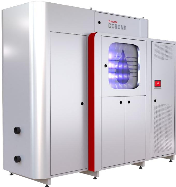
The first generation Flowrox Plasma Oxidizer is a 2-kW system, a single unit being capable of treating 1-25 m<sup>3</sup>/h depending on the application. The system is a plug-n-play unit with connection ports for inlet, outlet, drainage, and power. The treated water is fed from the top, allowed to pass through the plasma reactor and exit through the outlet port. The unit is illustrated in Figure 1.
