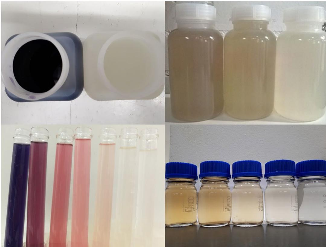
**Figure 2. Color removal by Flowrox Plasma Oxidizer plasma treatment. Left: textile industry wastewater; top right: high turbidity industrial wastewater; bottom right: biologically treated wastewater effluent.**
