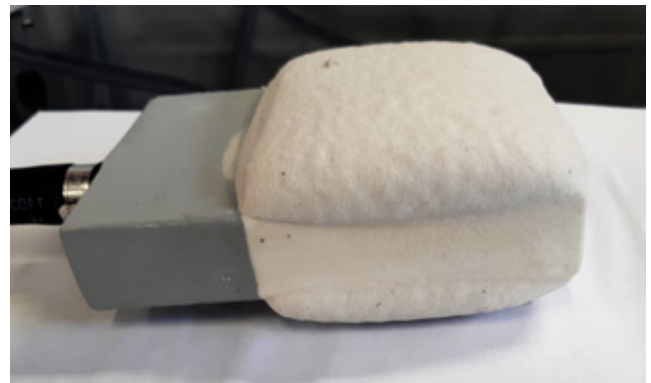
Ceramic plate before (left) and after (right) cake formation. The test simulates the operation of the full-size industrial filter.
