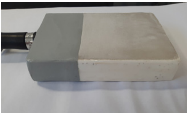
Ceramic plate before (left) and after (right) cake formation. The test simulates the operation of the full-size industrial filter.
