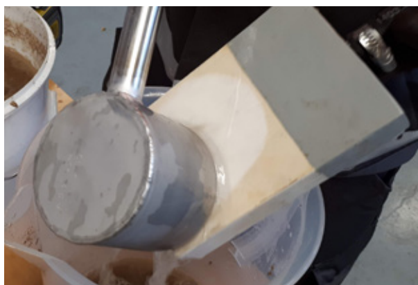
The ceramic disc test unit can also simulate the ultrasonic washing cycle just like the full-size industrial filter
