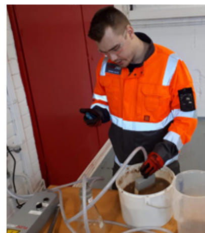
Simple ceramic dip test set fits in a smaller suitcase and requires little space.
