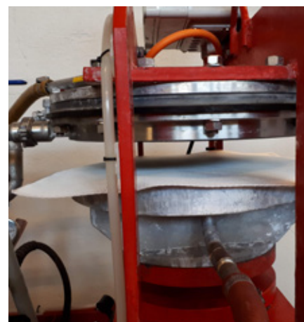
Tower press test unit simulates the operation of the full-size industrial filter.
