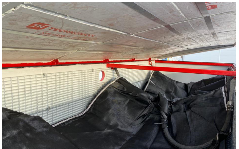
The geotextile filtration bag is mounted inside the container.
