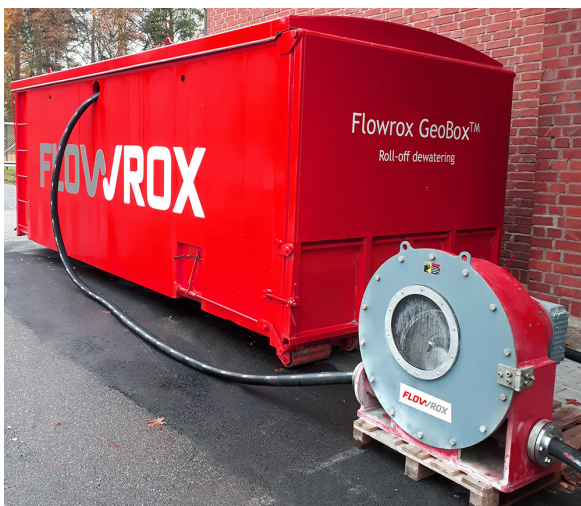
Outside view of Flowrox GeoBox™ with an LPP-T2.5" sludge transfer pump.
