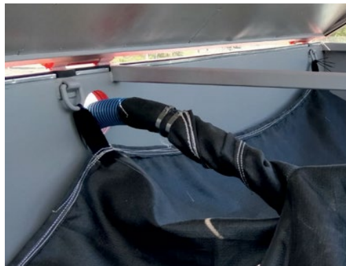
Geotextile bag sleeve is wrapped and fastened around the sludge inlet. Sludge feed through container inlet port.
