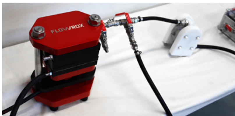
Filter press test unit simulates the operation of the full-size industrial filter.
