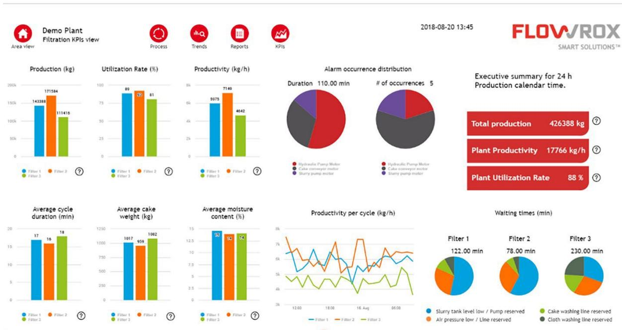
Figure 5. KPI chart developed with input from customer to display key performance indicators as well as alarms on the machines.
